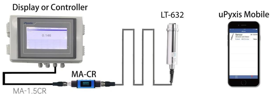
Figure 5 - LT-63X Series Sensor and MA-CR Bluetooth Adapter Powered By Connected Display, Controller or PLC
